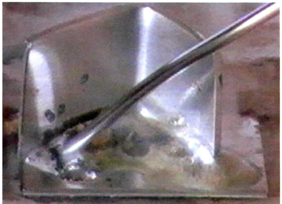
Fig. 6 — Soldering aluminum to aluminum with a soldering filler metal containing cored flux.
