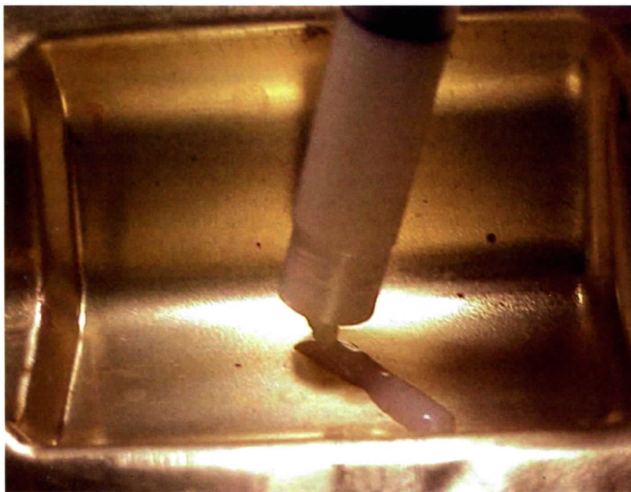
Fig. 4 — Paste flux dispensed to a metal surface.
