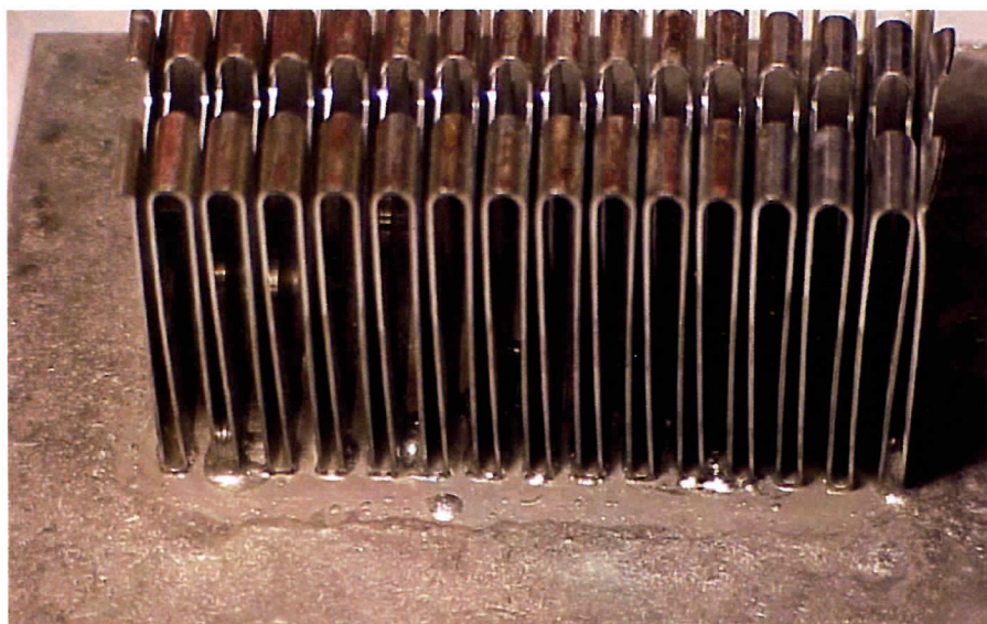
Fig. 3 — After hot plate heating, the soldering filler metal has flowed and connected the aluminum parts.
