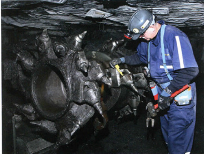
A miner changes conical bits on a continuous miner. (Photo courtesy of Kennametal)
