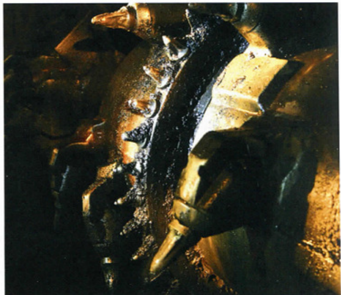
Cemented carbide bits are brazed to a steel shank. (Photo courtesy of Kennametal)
